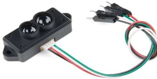
Fig.2. TFMini – Micro LiDAR sensor
